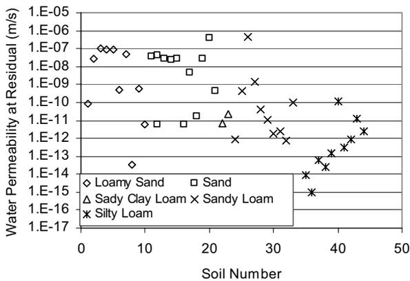
Figure 2. Computed coefficients of water permeability at residual conditions for water permeability predictive procedure proposed by Fredlund et al., 1994
