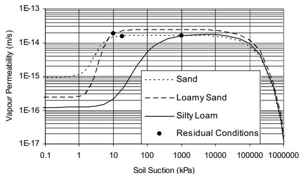
Figure 4. Vapour permeability curves for three soils.
