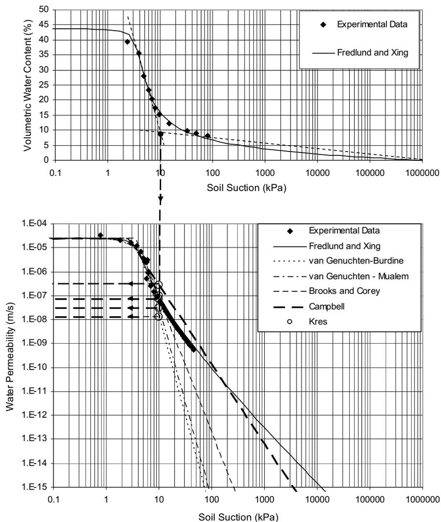
Figure 1. a) Fredlund and Xing's soil-water characteristic curve for loamy sand and b) Various water permeability models for loamy sand and water permeability at residual water content for each model (soil counter: 11178, SoilVision 3.34)
