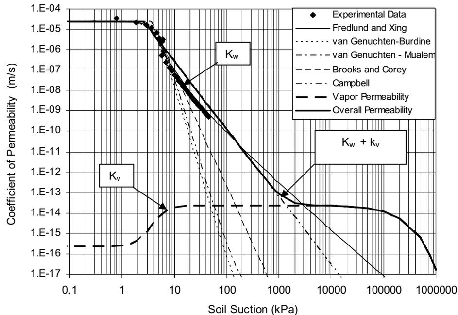
Figure 5. Variations of liquid water, vapour, and overall permeability coefficients with soil suction for a loamy sand soil
