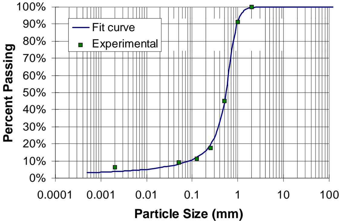
FIGURE 4 Grain-size distribution curve fit for a sand (#10720).
