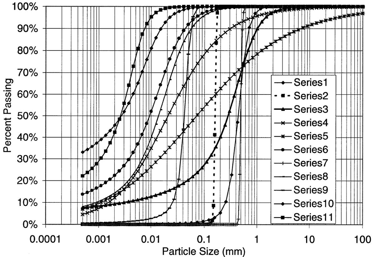
FIGURE 7 Theoretically fitted grain size curves for 11 soils.
