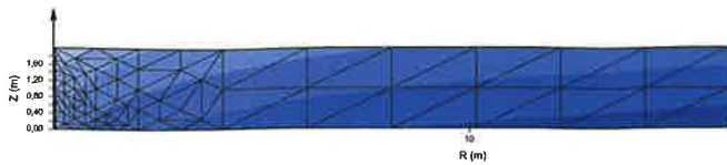
Figure 3. Pumping well (confined aquifer) model geometry with mesh generated by adaptive mesh generator; take a note that few triangles have an angle higher than 90 degrees, which means a poor shape for calculations (axisymmetric problem, radius of confined aquifer was 600 m).
